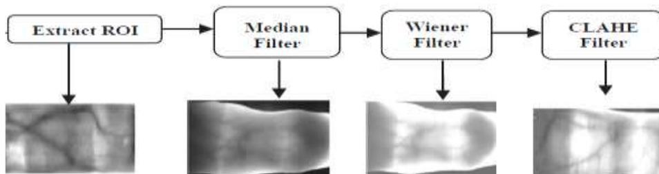
Fig. 6. The steps of preprocessing of finger veins
