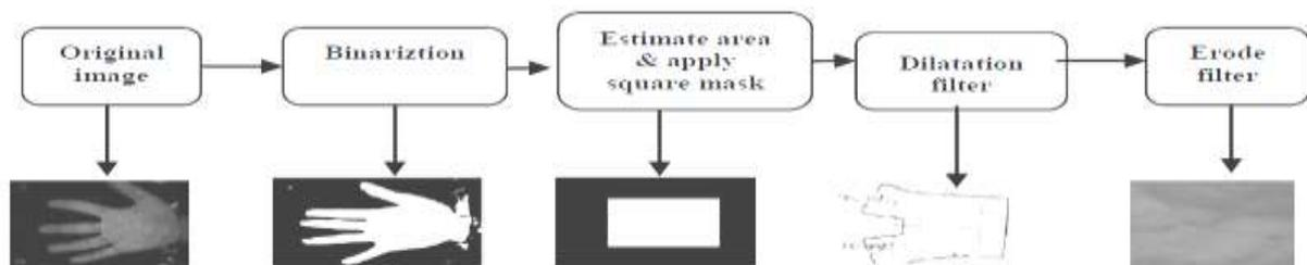
Fig. 3. The steps to detect ROI of palm veins
