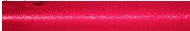
Fig. 9. Longitudinal beam track with high levels of contamination
