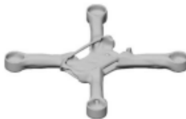
Fig. 6. Result of body geometry optimization
