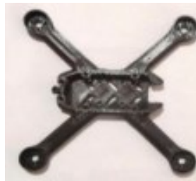
Fig. 3. UAV frame manufactured by 3D printing
