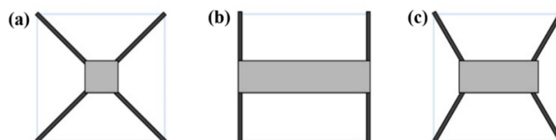
Fig. 1. Types of quadcopter frames: (a) Plus-shaped; (b) H-shaped; (c) X-shaped
