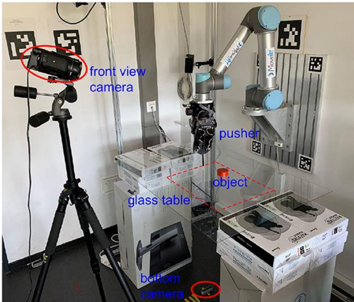
Fig. 2. Robot detects the objects and works with them
