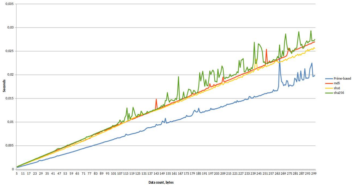
Fig. 5. Median of elapsed time to get 100 prime-based spectral Bloom filters
